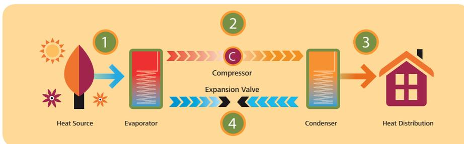
**1** A heat exchanger contains refrigerant, which is colder than the outside air. As the air passes the exchanger, the refrigerant absorbs the latent heat from the outside air and evaporates.
