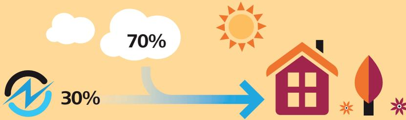
A heat pump simply moves heat, extracting the latent heat from the outside air and transferring it into the
