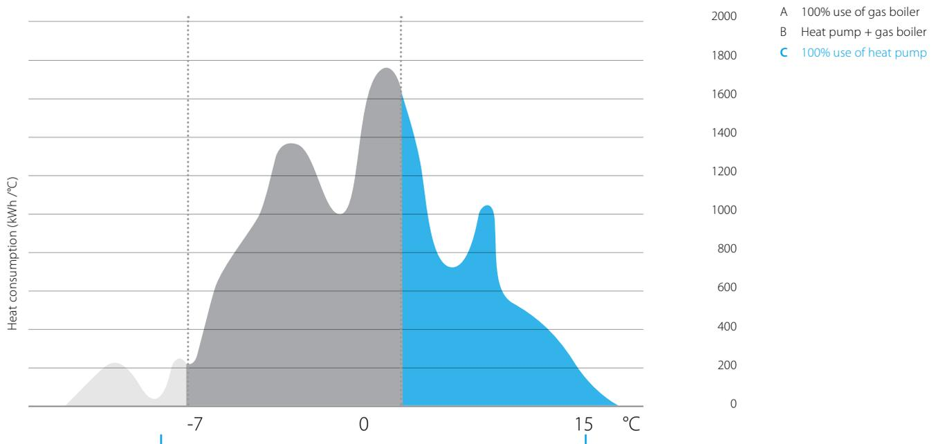
**+35% efficiency (space heating) compared to existing condensing gas boiler**
